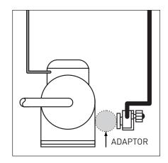
**GENERAL** – The oil level adaptor kits described below are used to attach the Sporlan oil level control to the sightglass connection on the compressor housing. In addition to the adaptor fitting, the kits contain the necessary bolts, nuts, O-ring, and sightglass (except AOL-R-1). All Sporlan oil level controls have the same 7 bolt universal flange connection. The adaptor kits permit installing the oil level control onto compressors with various threads or mounting hole configurations.
